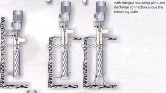
NEMO® Semi-Submerged Pump BT with integral mounting plate and discharge connection below the
