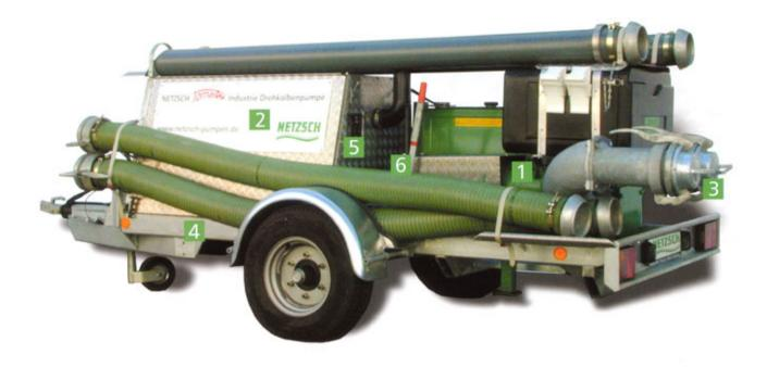
1 Pump Typ XLB4-JD-60kW bi-directional, self priming rotary lobe pump, pulsation free helical lobes made from GG25 cast iron with NBR rubber coating. Bearings only on drive side to allow quick lobe replacement, adjustable housings,
